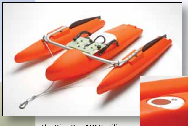
The RiverRay ADCP utilizes a flat-surface, phased array transducer.
