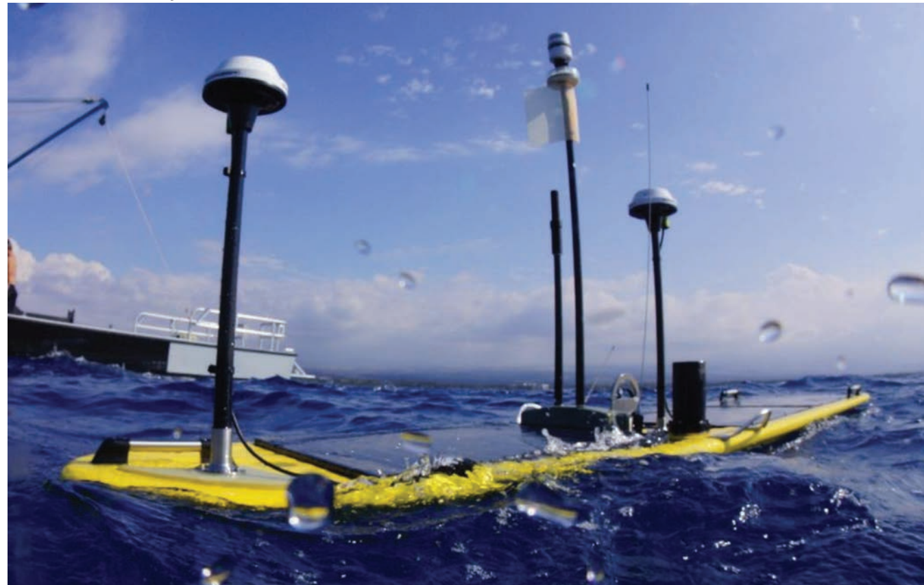
The surface part of a Wave Glider is a surfboard-like float that carries most of the payloads. Seen here is a float customized for a multibeam-sonar survey of the seabed.
