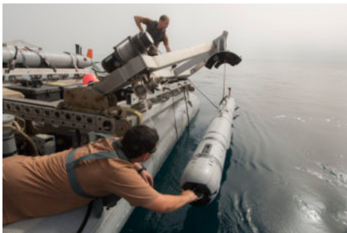
Sailors unload an underwater unmanned vehicle during mine countermeasures training operations aboard the USS Ponce (AFSB(I)-15)
