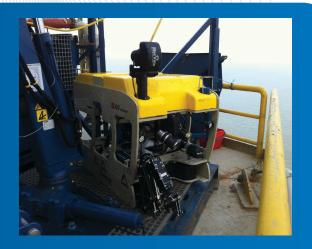
The highly portable, lightweight BlueView BV5000 is easily lowered into position around complex strucutres, or in remote, hard-toreach areas from waterside structures or small surface vessels. When combined with BlueView's lightweight tripod the BV5000 weighs approximately 40 lbs., and is perfectly suited for oneman deployment and operation.
