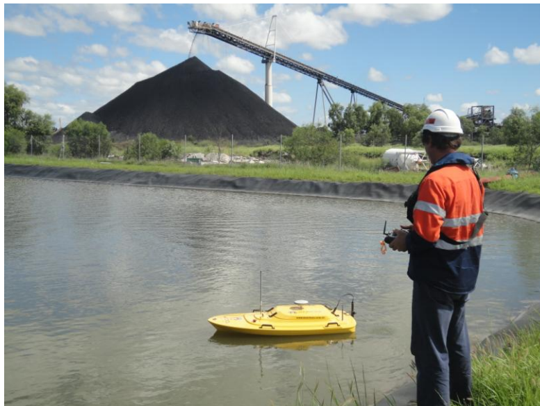
Figure 1. Z-Boat 1800 measuring sediment accumulation in Queensland, Australia.
