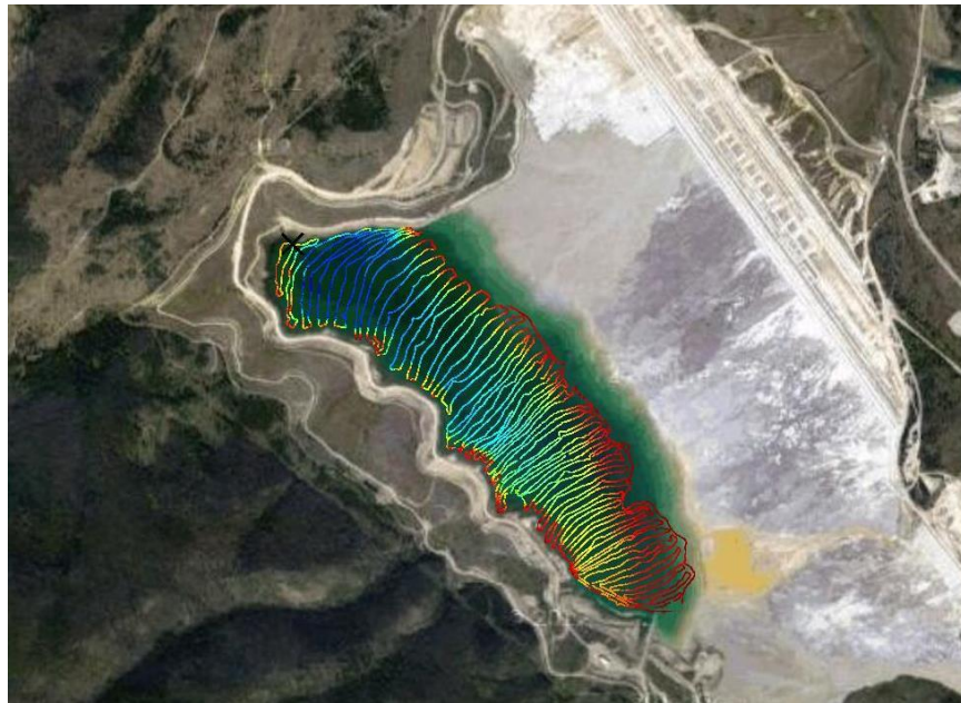
Figure 5. Z-Boat TSF survey completed in November 2012 using the Airmar DT800 with Trimble R8 GNSS.
