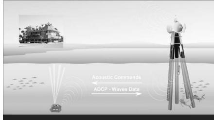
Wireless waves configuration: bottom mount, surface mount and repeater station on the beach.
