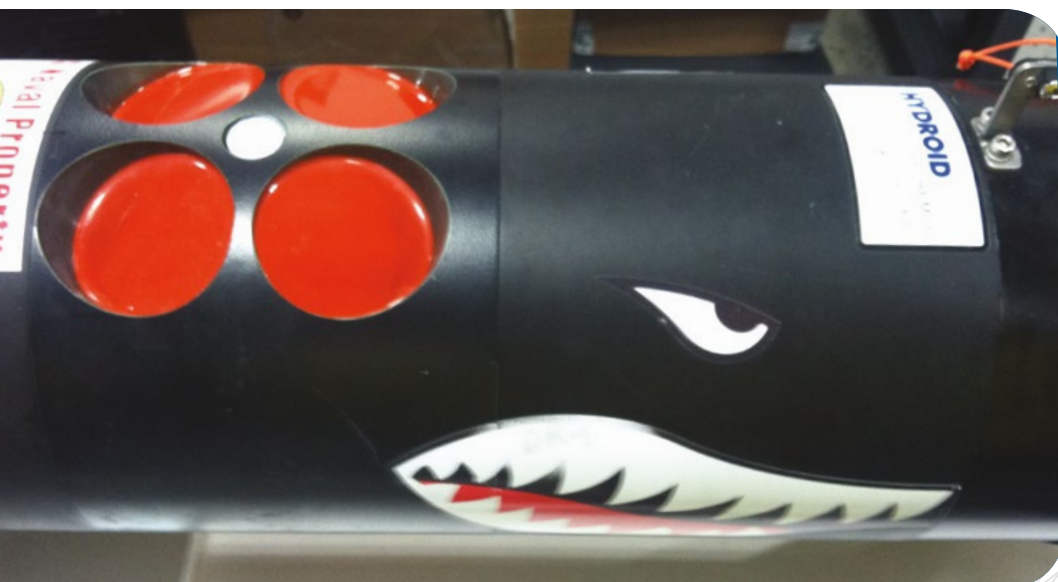
Hydroid REMUS 600, showing four faces of an uplooking ADCP. A matching set look downward.
