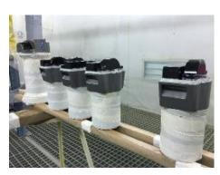
Coating of instruments with ClearSignal® biofouling control system is now underway at UVS workshops in Newcastle. Unlike anti-fouling systems that rely on active biocides and whose effectiveness degrades with time, ClearSignal® remains 100% effective for the intended life of the instrument.
