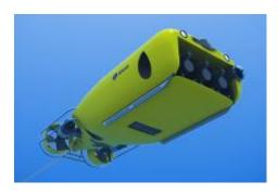
With a range of up to 1km and depth rating of 500m the Saab Double Eagle Mine Disposal System remains the reference system for remotely operated mine counter measures capability. Powerful propulsion packages enable underwater speeds of up to 8 knots ensuring that the Double Eagle can operate in the harsh maritime operational areas of Australia's coastal seas and oceans.
