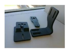
The BlueZone Group engineering team have kept the new Markforged carbon fibre / composite 3D printer busy at the Perth workshop. Printing continuously with Carbon Fibre, Fiberglass, and Kevlar the ability to produce printed parts with the strength of metal has turbo-charged hardware engineering development for BlueZone customers.
