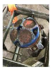
Rather than a spinning propeller, the Acoustic Doppler Current Profiler (ADCP) - like dolphins and bats - uses sound to explore its environment. Operating underwater, the method works like hand-held radars used by police to catch speeding motorists.
