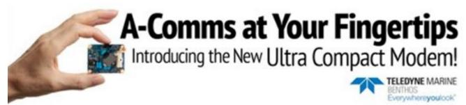
Teledyne Marine has announced the launch of its new Ultra Compact Modem (UCM). Sized at just 60mm x 50 mm, and weighing in at just 55 grams, the OEM version of the UCM is the smallest acoustic modem ever designed by Teledyne Benthos.
