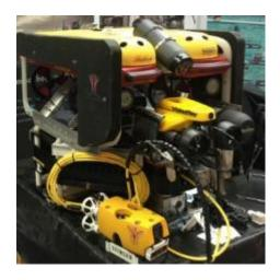
An ingenious idea from Saab Seaeye customer, Stinger Technology, has found a way to penetrate the labyrinth inside offshore production tanks in search of environmental contaminates prior to decommissioning. They managed to squeeze a unique underwater robotic systems configuration loaded with sampling technology through a 150 cm square hatch to search the tank's internal maze of baffles, and navigate along 25.5 cm diameter pipe-runs of curves and bends.
