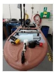
The Wave Glider SV3 v300 supports 30% heavier payloads with larger float interior and no change in external dimensions
