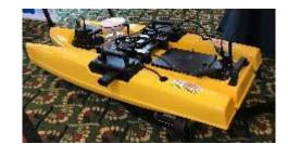
Teledyne OceanScience has announced the release of the new Z-Boat 1250, a remotely operated hydrographic survey boat that is sturdy enough for tough terrain but light enough to be one person portable. The new Z-Boat 1250 is outfitted with a single beam echo sounder and is ideally suited for inland waters such as streams, rivers, and lakes.
