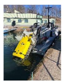
Saab's unique Multi-Shot Mine Neutralisation System (MuMNS) is a powerful, reliable and adaptable vehicle that can be used in a variety of different roles, including live operational mine clearance, peacetime operations against historical ordnance, mine investigation and underwater demolitions. The system is effective against a complete range of underwater targets: mines (ground, moored, floating and drifting), depth charges, torpedoes and IEDs.
